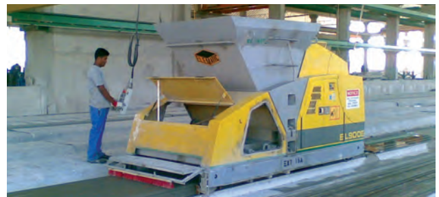
Extruder machine for production of hollow core slabs
